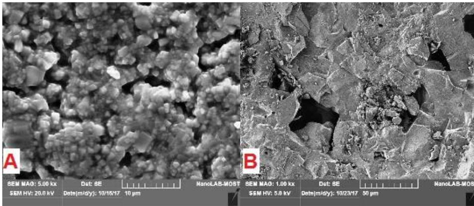
Figure 3. Scanning electron microscopy images show structural morphology of eggshell hydroxyapatite at (A) 500× (B) 1000×.
