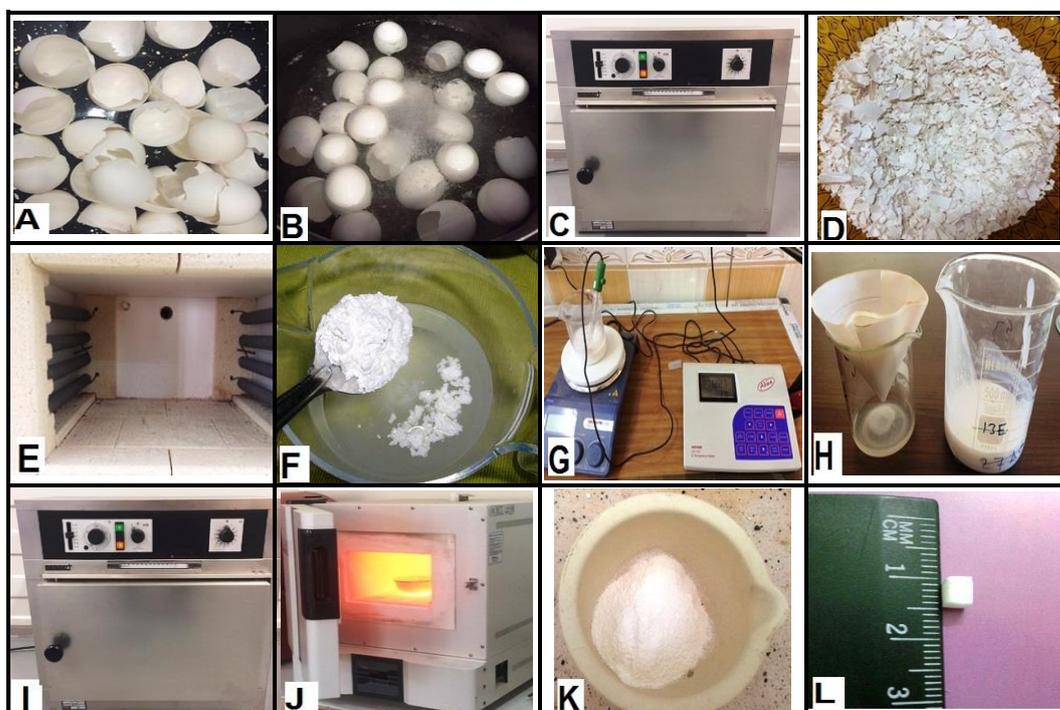
Figure 1. Synthesis of eHA (A), Cleaning and washing of egg shells (B), Boiling of egg shells in distilled water for 30 min (C), Drying in oven at 100c° for 30 min. (D) Crushing egg shells (E), Calcination at 1200 c° for 2 hr. (F) Dispersion of powder in water (G), Addin drops of H<sub>3</sub>PO<sub>4</sub> to adjusted PH to 8.5 (H),
