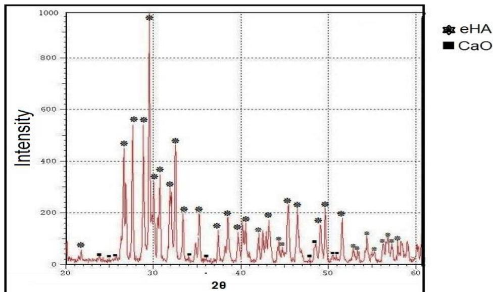
Figure 2. X- ray diffraction of eggshell hydroxyapatite intensities at scattering angles of  $2\theta$ .
